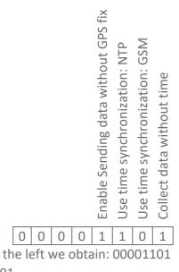
Reading register values from the left we obtain: 00001101 Number in binary format:  $1101_{BIN}$ Number in decimal format:  $13_{DEC}$
